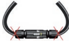
Incorrect routing of cable
