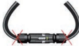
Incorrect routing of cable
